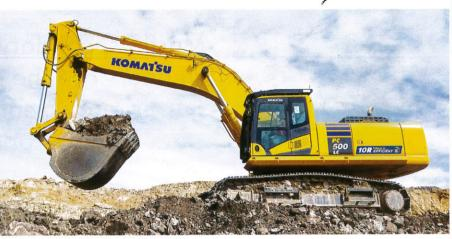
extended. This achievement is due to the specialised metallurgy used in the hydraulic components, which minimises wear and extends component life. In addition, Komatsu has developed a new hydraulic filter using nanotechnology, extending the filter change interval from 1000 to 2500 hours. This innovation reduces maintenance costs and environmental pollution.
